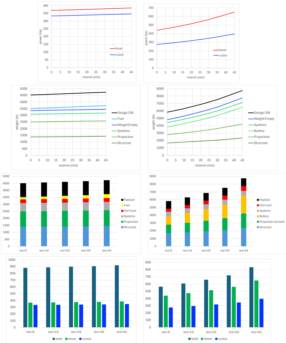
Figure 23. Quadrotor, turboshaft (left) and electric (right) — impact of mission reserve. The baseline design mission has a reserve of 20 min, corresponding to visual flight rules (VFR) rotorcraft operations. The reserve segment time is varied from 0 to 45 min.
