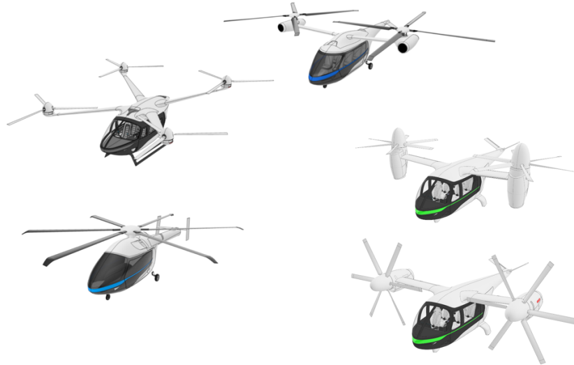
Figure 2. Aircraft for investigation of technology and mission variations: Quadrotor (quad), quiet single main rotor (QSMR), side-by-side (side), and tiltrotor (tilt) aircraft.
